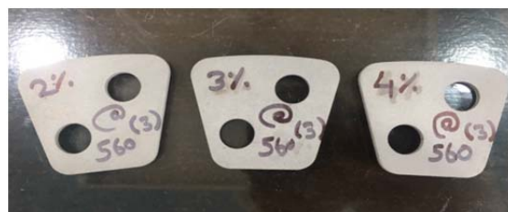
Fig. 4 Sintered FGM plates
