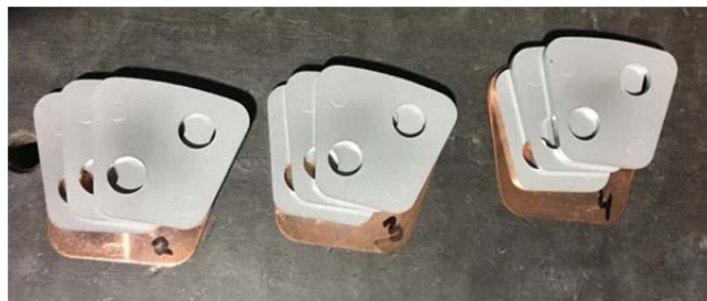
Fig. 3 Compacted FGM plates
